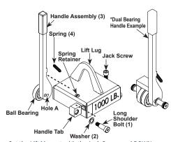
Set the Lift Magnet with the Jack Screw end DOWN, on a non-magnetic surface with the Handle Tab end UP in a vertical position.
