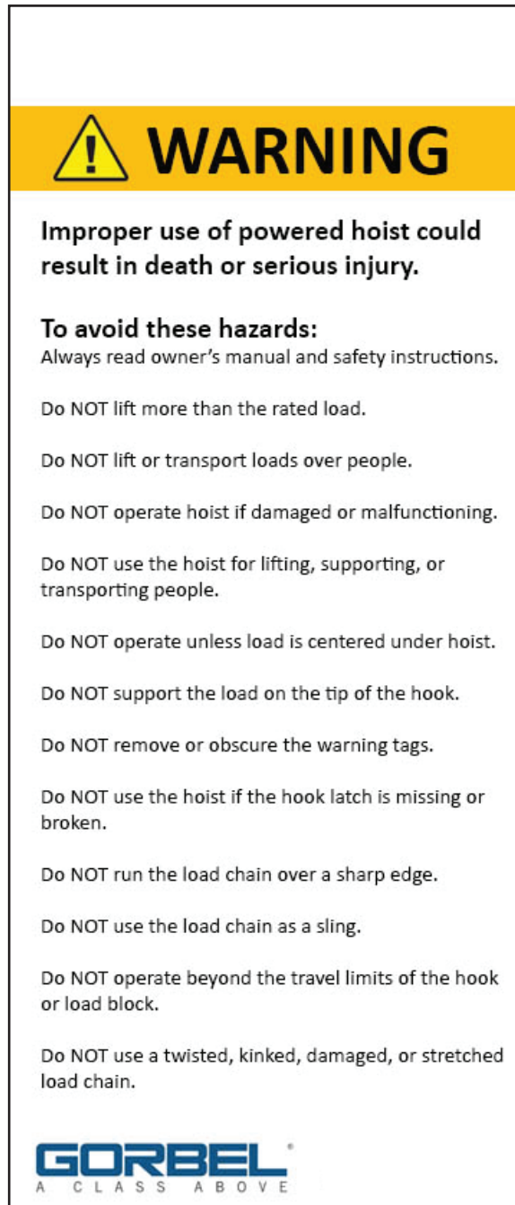
Figure 1: Warning tag on the control cable.
