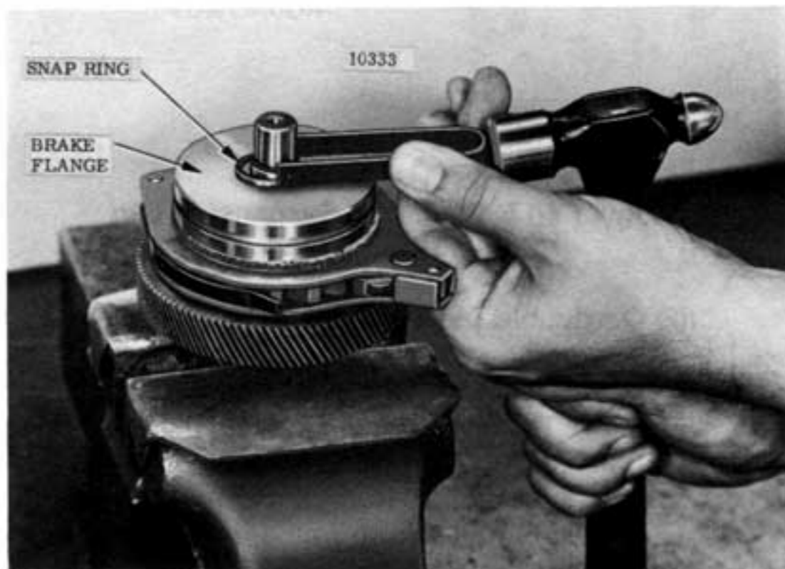
Figure 7-18. Removing Snap Ring from Load Brake Shaft.
