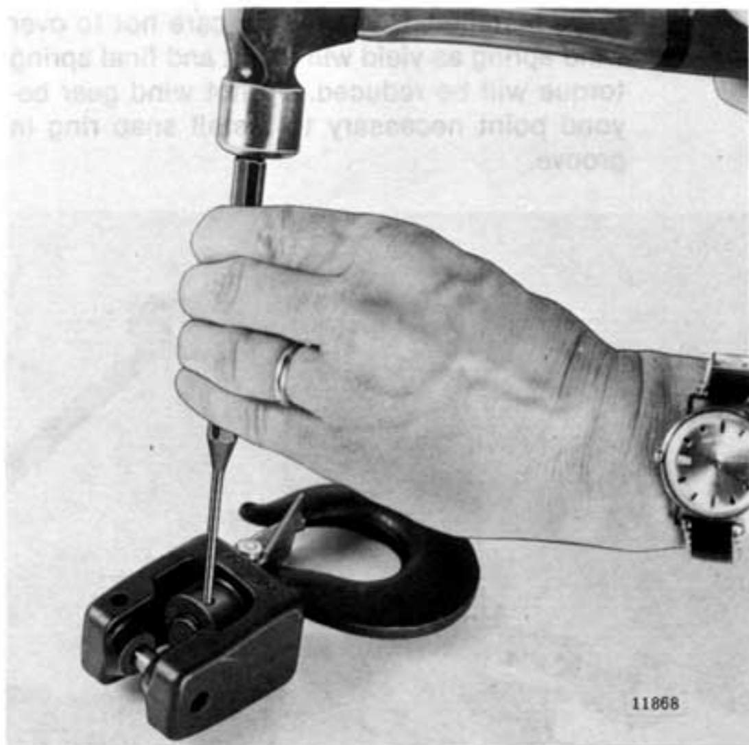
Figure 7-23. Removing Roll Pin Securing Hook Nut to Hook Shank.
