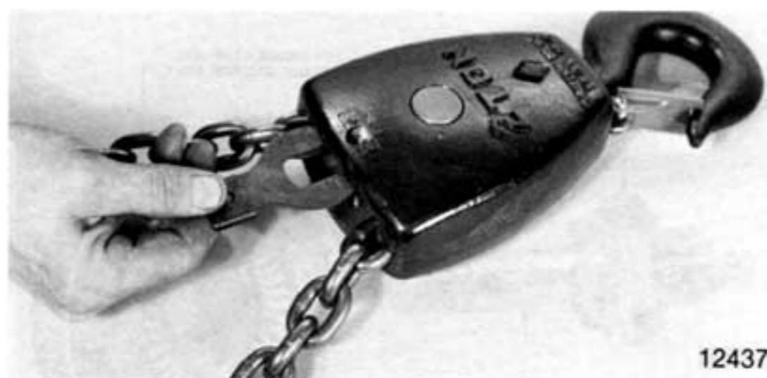
Figure 7-25. Removing Sprocket Pin Lock On Double and Triple Reeved Lower Block Assembly.
