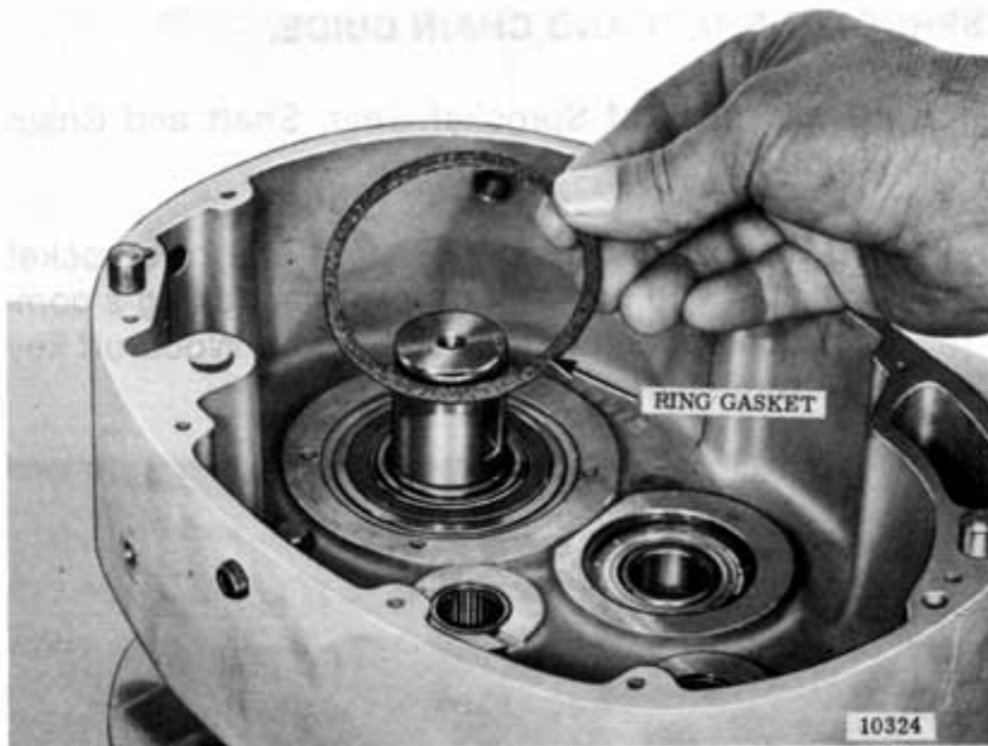
Figure 7-11. Removing Sprocket Bearing Ring Gasket. (On later model hoists ring gasket is replaced by a seal disk with oil seals.)
