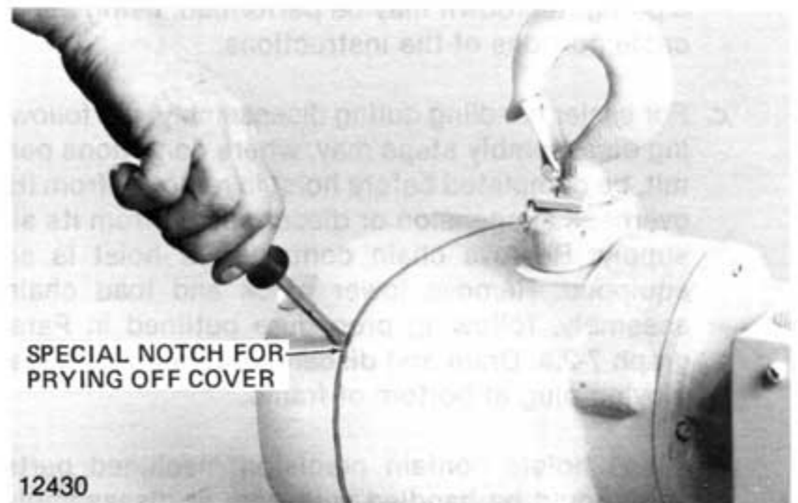
Figure 7-4. Prying Gearcase Cover From Hoist Frame.
